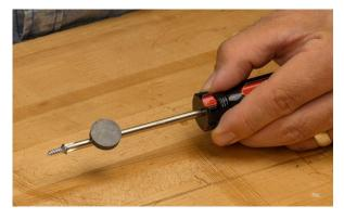
Magnetize the end of a screwdriver to drive screws with just one hand. This hint is especially useful for working in tight spaces where there isn't room for you to hold a screw with one hand while you turn the screwdriver with the other.
