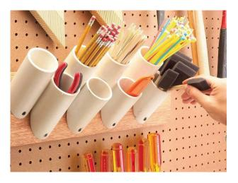
A few bits of poly pipe can be easily turned into useful containers for pens/pencils/brushes, screwdrivers and other small tools, etc. Cut at an angle and just screw on to a board or the wall - an easy and cheap fix.
