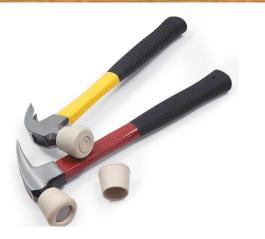
A rubber chair leg cap instantly converts a hammer into a rubber mallet. And if you want to drive a nail without denting the surrounding wood, cut a hole in the rubber cap. Pound until the rubber strikes wood, then finish driving the nail with a nail set. A 3 cm. rubber cap generally fits tightly over most hammers and costs just a couple of dollars at hardware or discount stores.
